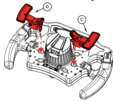
To prevent scratches place a finger on the magnet while tightening the screw.
