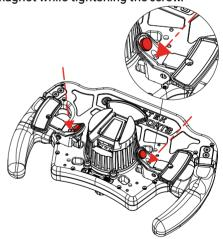
Adjust the shifter paddles to your preferred length, then securely tighten the screws.
